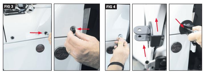
It is not necessary to remove the front doors to install the mirrors, but adjusting the mirrors will be much easier if the doors are removed. Remove the Torx bolt using a T40 Torx bit driver or Ratchet. (Fig 3) Place one steel spacer as shown. Align the bracket to the inner A-pillar and push the bracket towards the front of the vehicle. Use one Torx bolt, one plastic washer and tighten the bracket with a T40 Torx bit or ratchet. (Fig 4)
