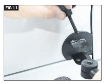
To remove the mirror, loosen the adjustable knob from the bracket. Remove the knob and the mirror. Store the mirror in a safe place. (Fig 11)
