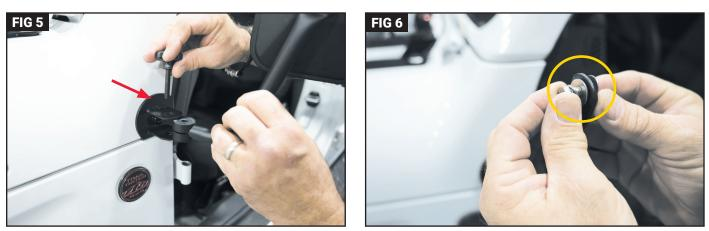
Place one mirror arm into the bracket. Attach one adjustment knob through the bushing on the mirror arm. (Fig 5) Remove the hardware attached to the mirror. Place one bolt, one lock washer and one flat washer through the top of the mirror arm followed by the second flat washer on the other side of the arm. (Fig 6)
