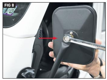
Thread one M8 bolt into the mirror mount through the mirror arm. (Fig 7) Tighten the bolt to the mirror through the top arm using a 12mm wrench. (Fig 8)
