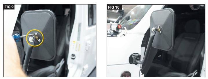
Adjust the mirror to the desired position using a phillips head screwdriver. DO NOT OVER TIGHTEN phillips head screws. The mirror should not be so tight that it cannot be adjusted. (Fig 9) Installation is now complete. Repeat steps 1 through 4 for the other side. (Fig 10)
