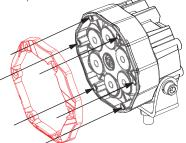
**3.** Take 6 of the M4 bezel screws (#1), place them in the holes of the outer bezel, and fasten the lens and bezel to the light using the T20 Torx Wrench. Repeat steps 1-3 on the other light.
