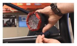
**12.** Aim the Trail 6 as desired and fasten the side bolts (#5) using 5mm Hex Key. Plug in the provided daisy chain harness into the back of the lamp.
