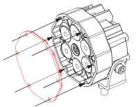
**2.** Place the outer bezel (#2) on the lamp over the lens. Be sure the J.W. Speaker logo on the outer bezel is oriented at the bottom of the lamp.
