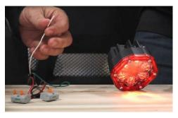
**OPTIONAL:** Splice the white **Brake Override** wire with your brake wire. This will cause the Trail 6 Flash to work with your brakes. **If unused, cap the white wire.**
