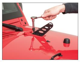
With the Factory bolts removed install the Driver and Passenger brackets as shown with the supplied M8 T40 Torx
