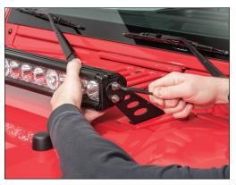
While supporting the light bar parallel to the hood install the 6mm socket headed screw, lock washer and flat washer through the hole in the bracket and thread it into the light bar. Install another 6mm socket headed screw, lock washer, and flat washer into the slot on
