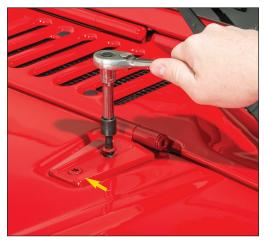
ratchet. (it may be necessary to score the paint around the bolts using and razor blade to prevent paint chipping.)
