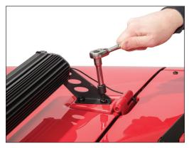
the bracket. Continue to support the bar and repeat on the opposite side. Snug the cap screws with a 5mm hex key but do not fully tighten at this time. Fully tighten the hood fasteners at this point with a T40 bit and ratchet.
