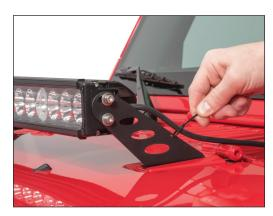
Route wires as needed. Please refer to the light bar and harness instructions provided with those components. The slots on both brackets can be used to secure the wires using the supplied zip ties as shown.
