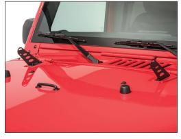
bolts and nylon washers. Snug but do not fully tighten the bolts using a T40 Torx bit or key.
