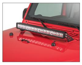
Adjust the light bar to the desired angle and then fully tighten all 4 socket headed screws with a 5 mm hex key.
