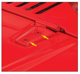
Put on Safety Glasses. With the hood securely latched in place, locate the two T47 Torx bolts on both hood hinges and remove them using a T47 Torx bit and
