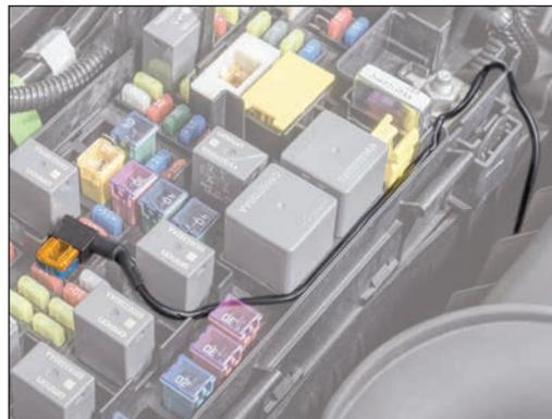
*Install the fuse holder back into the M18 fuse location in your fuse box. Route the wire as show and replace the fuse lid. Be careful not to pinch the wire.*
