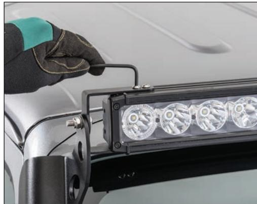
*Snug the button headed screws on the top and bottom of both ends of the lightbar with a 4mm hex wrench.*
