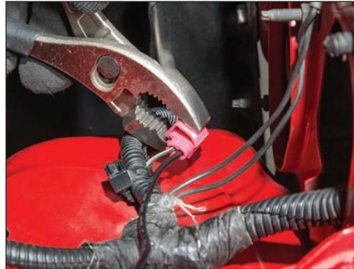
*close and latch the cover wing of the wire tap to complete the circuit. For best weather resistance, wrap the wire tap with black electrical tape. (not shown)*
