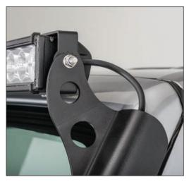
The main power wire can be routed behind or next to your A pillar mounting brackets.
