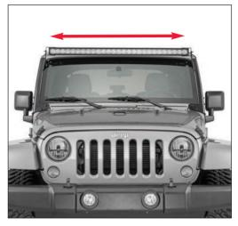
Position the light bar on your mounting brackets and center it left to right on your the vehicle.
