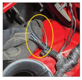
senger front corner of the vehicle. Locate the wire loom behind headlight bucket and extract the black wire with yellow tracer stripe.
