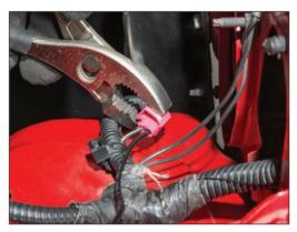
close and latch the cover wing of the wire tap to complete the circuit. For best weather resistance, wrap the wire tap with black electrical tape. (not shown)
