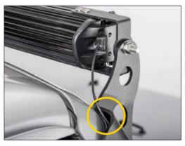
The Clearance light accessory wire can be routed behind or next to your A pillar bracket.
