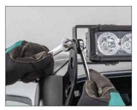
Attach the light bar to your brackets with the provided bolt, nylock and washer. Tighten the nut and bolt with two 13mm wrenches or a wrench and a 13mm socket.
