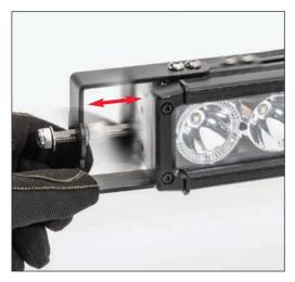
Put on Safety Glasses. Loosen the button head hex screws (4) on the top and bottom on each end of the light bar brackets with a 4mm hex key. This will allow the brackets to slide in and out in order to fit multiple width light bar mounts.
