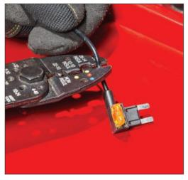
On TJ vehicles: Snip off the fuse tap on the end of the accessory wire on your new lightbar. Route the wire under the hood along the fender wall to the pas-
