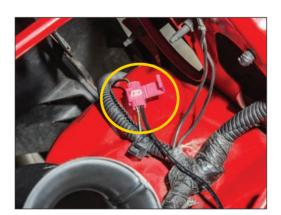
Install the supplied wire tap over the black wire with yellow tracer stripe. Install the cut end of the accessory wire into the other slot in the wire tap as shown. Using your pliers, gently
