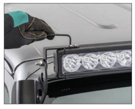
Snug the button headed screws on the top and bottom of both ends of the lightbar with a 4mm hex wrench.
