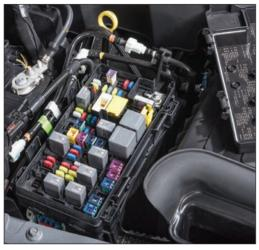
On JK vehicles: The fuse box is located under the hood on the right hand side of the engine compartment. Locate fuse panel lid and remove it.
