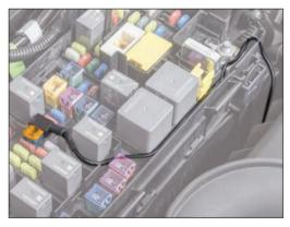
Install the fuse holder back into the M18 fuse location in your fuse box. Route the wire as show and replace the fuse lid. Be careful not to pinch the wire.
