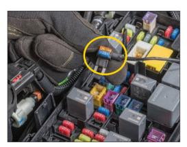
Remove the 15 amp fuse and install it in the lower slot of the light bar harness fuse holder. The upper slot should have a 5 amp fuse pre-installed in it.
