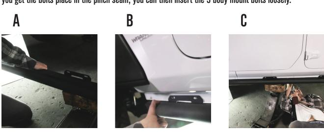
4 Next, remove the jack and begin tightening the bolts. Start with the 6 bolts that go through the pinch seam. Use a 3/16 Hex and a 13mm end wrench to tighten the pinch seam bolts. Next, tighten down the 3 body mount bolts with the 18mm socket.
