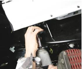
Begin to install your new JCR Slider. Use a jack to hold the slider in place as you insert the bolts. Once the holes are lined up with the pinch seam, loosely place the bolts through the holes. Once you get the bolts place in the pinch seam, you can then insert the 3 body mount bolts loosely.
