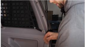
96 -: You will not have this interior screw. Install the rear bracket on the MOLLE panel and use the rear hole as a guide. Drill through the interior plastic and the sheet metal behind it. Install using the provided sheet metal screw.
