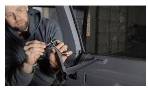
**3** Put the MOLLE panel in place, behind the seatbelt and in front of the mounting brackets. Loosely bolt it in place.
