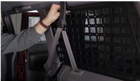
4 97 +: Remove the interior panel screw as shown and reinstall through the rear MOLLE panel bracket using the supplied screw. The bend will go towards the MOLLE panel.
