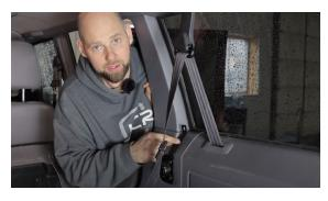
2 Remove the upper seatbelt bolt using a T-50 Torx. Place the upper MOLLE panel bracket over the seatbelt bracket as shown. Reinstall the bolt & brackets, ensuring that the tab on the seatbelt bracket is up inside the roof.
