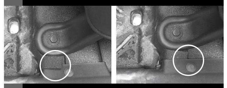
Ensure the wires located under the seat are fed between the cut slots in the Armorlite floor, and that the hole in the Armorlite floor is over the post in the sheet metal. Make sure drain hole is aligned with the sheet metal hole before installing drain plug.
