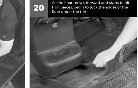
Repeat steps 19 and 20, by alternating sides until the rear Armorlite floor is in the correct position. Use the drain hole as a reference.
