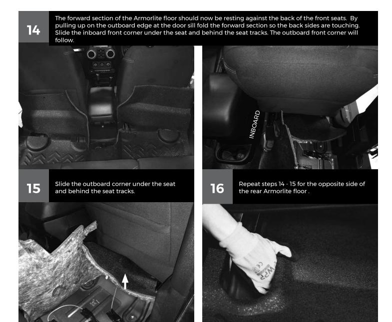
Tuck the outboard edge under the door sill. Ensure that the floor is tucked under the trim at the "B" pillar and NOT against the trim. This will result in an improper fit and the drain holes will not align.
