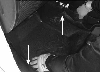
From front to rear start tucking the inboard edge under the center console trim at the point indicated in the picture.
