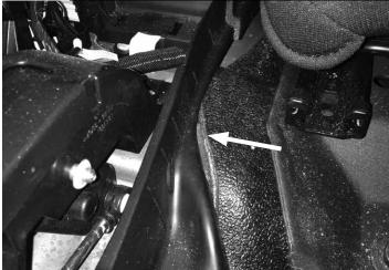
Tuck the outboard corner of the rear center flap under the seat, behind the seat track and under the door sill.
