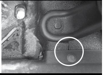
Ensure the wires located under the seat are fed between the cut slots in the Armorlite floor, and that the hole in the Armorlite floor is over the post in the sheet metal. Make sure drain hole is aligned with the sheet 9 metal hole before installing drain plug.
