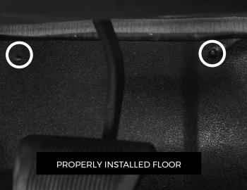
Pull up on the inboard edge of the Armorlite floor, as you tuck the outboard edge under the door sill trim.
