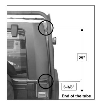
(Step 22) Secure each end of the Cargo Cross Bars to the top of the Side Tubes with (1) Fastening Bolt, (2) 8mm x 24mm STD Flat Washers and (1) 8mm Nylon Lock Nut.
