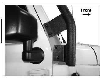
**(Step 4)** Select Front Main Cross Tube. Insert Cross Tube into passenger/right Front Rack Leg. **NOTE**: Cross Tube can be installed with light tabs to the front or rear.
