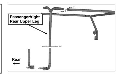
(Step 12) Select the Rear Main Cross Tube. Insert Cross Tube into passenger/right Rear Upper Rack Leg. NOTE: Cross Tube can be installed with light tabs to the front or rear as desired.
