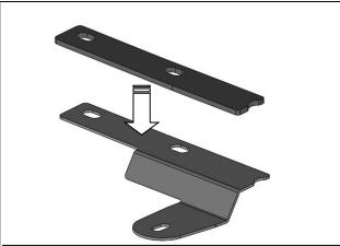
(Fig 1) For models with a hardtop, attach (1) Long Foam Strip to the top of the Driver/Left Front Bracket
