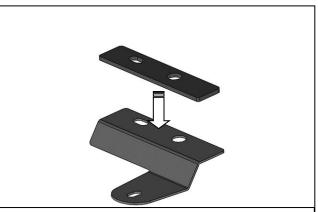
(Fig 3) For models with a hardtop, attach (1) Mid Foam Strip to the top of the Driver/Left Rear Bracket
