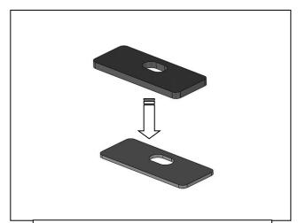
(Fig 2) For models with a hardtop, attach (1) Short Foam Strip to (1) Spacer Plate
