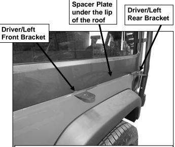
(Fig 5) Lift the hardtop and place the Driver/Left Brackets and (1) Spacer Plate under the window. Line up the holes in the brackets to the holes in the roof used for the bolts
