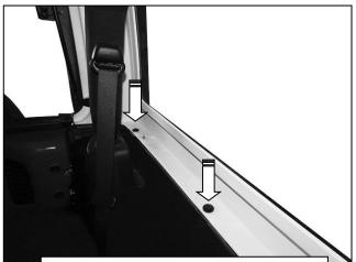
(Fig 4) Temporarily remove the (6) bolts attaching the hardtop roof to the vehicle. Place bolts in a safe location
