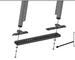
(Fig 6) Attach (1) Left Accessory Tube, (1) Right Accessory Tube and (1) Step Pad to the Driver/Left Brackets
