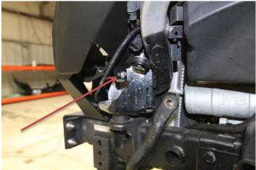
**10.** Fully tighten the remaining three bolts. Two bolts under the hood and one bolts on the pinch weld under the door.
