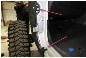
**9.** The third bolt to be tightened will be the front most bolt. Pull the nose of the fender out and away from the frame as much as possible and filly tighten the bolt that is located inside the wheel well and behind the headlight.
