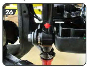
x. Install the remaning longer sleeve on the driver side and slide the polyurethane spacer onto the sleeve so it will mount towards the axle mount tab. Install the quicker disconnect to the inboard side of the axle tab with the original sway bar link hardware.
