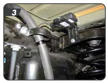
Rubicon models: Disconnect the locker wires from the differential.
