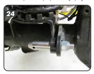
q. The kit comes with disconnect retention brackets to hold the links when the links are disconnected. Install the retention brackets using the provided 5/16" bolts into the factory hole in the front of the coil bucket [25]. These are designed to slightly interfere with the edge of the coil bucket to hold them in place.
