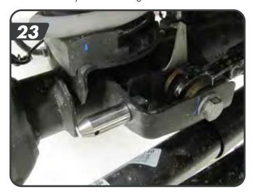
p. Install the longer disconnect post on the driver side axle sway bar link mount with it pointing inboard [24]. Fasten with the ½" nylock nut and tighten to 64 ft-lbs. Tighten the post with the pin hole parallel to the ground. Slide the polyurethane spacer on the pin up against the axle tab.
