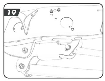
Note: it may be easier to align the control arms to the mount by removing the opposite side upper control arm adn adjusting the axle with a hydraulic
