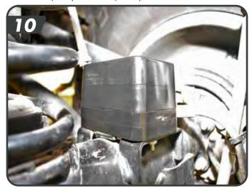
d. The shocks come with the bushings and upper spacers pre-installed. The wide mount will be installed up, at the frame. Slide the shock up into the mount. JSPEC shocks will be installed body down, Fox shocks will be installed body up.
