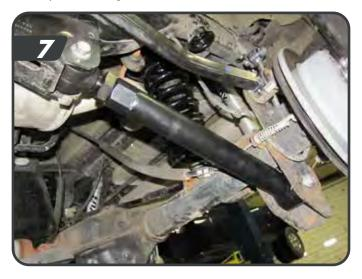
n. Mount the control arm to the frame bracket with the grease fitting up. Install the original mounting bolt and flag nut. Finger tighten the bolt. DO NOT torque mounting hardware until instructed.
