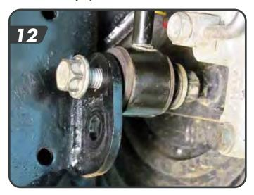
Install the rear bump stop spacers on the axle with the 2'' tall orientation for 2.5'' lifts and 3'' orientation for 3.5'' lifts.In both cases the bump should be intalled with the offset in material forward. Fasten the bump stop spacer to the axle with the  $5/16" \times 7/8"$  bolts, nuts and washers. Torque bolts to 20 ft-lbs. (½") [13]
