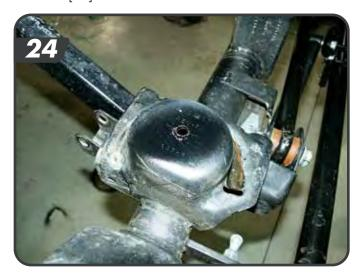
ab. Place the provided bump stop extension inside one of the JSPEC front coil springs. Note: Taller springs are for the front. Install the front coil springs with the bump stop extension. Make sure the spring is seated properly in the axle mount.
