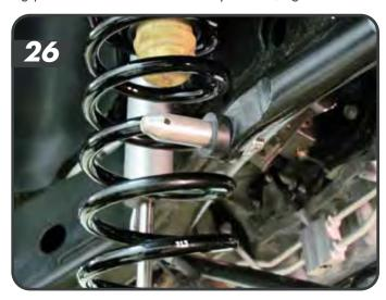
Note: A small screwdriver or punch inserted into the pin hole will keep the post from turning as you tighten it.
