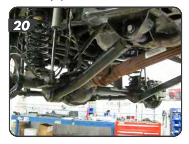
i. Mount the control arm to the frame rail bracket so the grease fitting is up on the flex eye. Install the original mounting bolt and nut. Finger tighten the bolt.
