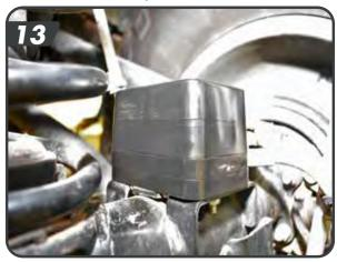
v. The shocks come with the bushings and upper spacers pre-installed. The wide mount will be installed up, at the frame. Slide the shock up into the mount. JSPEC shocks will be installed body down, Fox shocks will be installed body up.
