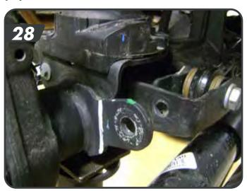
al. Install the shorter passenger side post on the side of the track bar mount at the sway bar link mount location with it pointing outboard [29]. Fasten with the ½" nylock nut and tighten to 64 ft-lbs.
