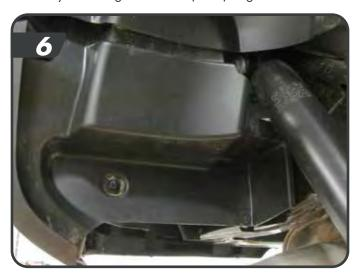
Support the axle with a jack under the center of the differential and remove the shocks from the frame and axle (18mm), save hardware [7].
