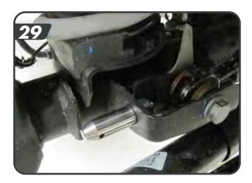
am. Install the longer disconnect post on the driver side axle sway bar link mount with it pointing inboard [30]. Fasten with the ½" nylock nut and tighten to 64 ft-lbs. Tighten the post with the pin hole parallel to the ground. Slide the polyurethane spacer on the pin up against the axle tab.
