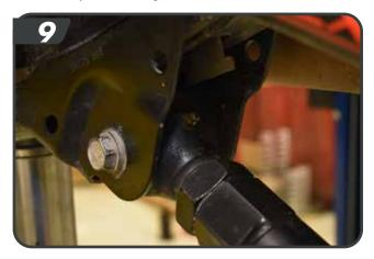
HINT: If mounting bolt is difficult to install due to misalignment of the control arm bushing with mounting bracket, either (1) adjust height of axle housing with hydraulic jack, or (2) move axle housing into position with a heavy-duty ratchet strap.
