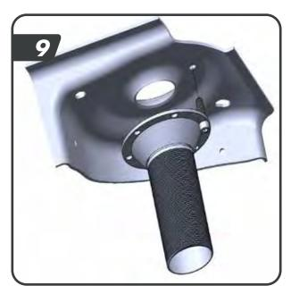
f. Using the Cone Adapter Plate as a template, accuratly mark the 5 remaining hole locations on the upper spring mount. *Hint: A transfer punch or similar tool is useful for marking hole locations.*  g. Remove the Cone Adapter Plate and drill a pilot hole at each marked locations using a ¼" drill bit. Enlarge each hole with a 3/8" drill bit. [10]
