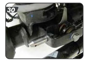
s. Install the longer disconnect post on the driver side axle sway bar link mount with it pointing inboard [31]. Fasten with the  $\frac{1}{2}$ " nylock nut and tighten to 64 ft-lbs. Tighten the post with the pin hole parallel to the ground. Slide the polyurethane spacer on the pin up against the axle tab.
