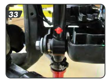
aa. Install the remaning longer sleeve on the driver side and slide the polyurethane spacer onto the sleeve so it will mount towards the axle mount tab. Install the quicker disconnect to the inboard side of the axle tab with the original sway bar link hardware.
