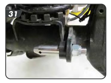
t. The kit comes with disconnect retention brackets to hold the links when the links are disconnected. Install the retention brackets using the provided 5/16" bolts into the factory hole in the front of the coil bucket [32]. These are designed to slightly interfere with the edge of the coil bucket to hold them in place.
