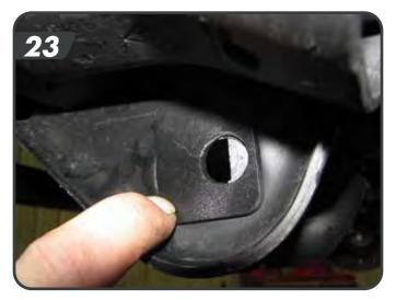
d. Re-install the control arm to the axle with the factory bolt with cam lock washers. Rotate the cam lock so that the bolt will be as far back in the slot as possible (most rearward setting = max caster). Snug the cam hardware so that the cams are retained within the stops. Final torque will be completed with the weight of the vehicle on the suspension. [24]
