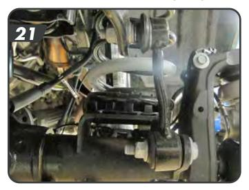
h. Remove the 4 bolts mounting the front driveshaft to the pinion flange (15mm). This is done to ensure the driveshaft does not bind when removing the coil springs. [22]
