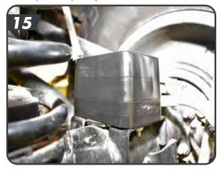
aa. The shocks come with the bushings and upper spacers pre-installed. The wide mount will be installed up, at the frame. Slide the shock up into the mount. JSPEC shocks will be installed body down, Fox shocks will be installed body up.
