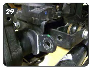
r. Install the shorter passenger side post on the side of the track bar mount at the sway bar link mount location with it pointing outboard [30]. Fasten with the ½" nylock nut and tighten to 64 ft-lbs.
