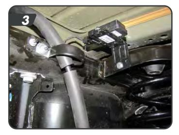
f. Rubicon models: Disconnect the locker wires from the differential.
