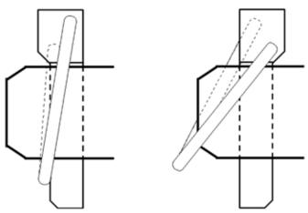
When properly installed, the ring on the Click Pin will "snap" against the shaft of pin. When installed backwards, the ring does not fit snugly against shaft.
