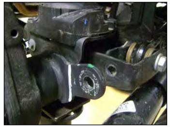
• Attach the short mounting post into the original sway bar link mount hole on the track bar bracket. Tighten the post ensuring the click pin hole is horizontal or parallel with the ground. Tighten to 65 ft-lbs.
