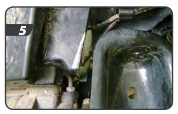
The bottom of the plastic tray must be trimmed to provide clearance for the coilover bracket. Test the bracket fitment by temporarily holding up the main coil-over mount to the frame and lining up the OE brake line mounting hole to the lower hole in the bracket. Clearance as necessary. [6,7]
