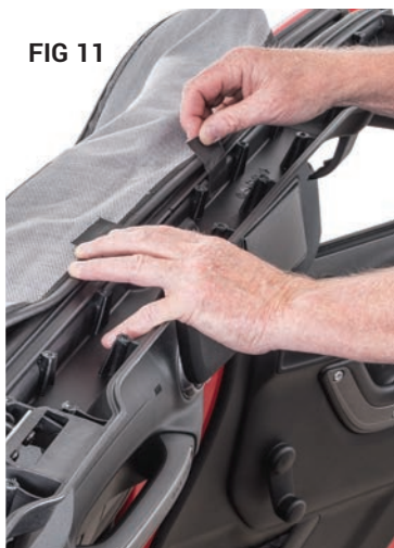
Once centered, use a heavy masking tape on each side of the notch to hold in place.
