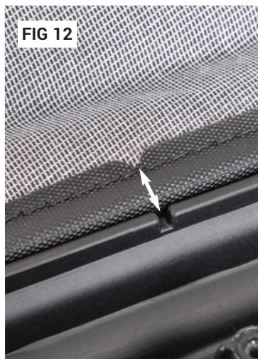
Center notch in fabric with the notch in the header.
