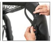
Thread the straps down and under the seat belt mount as shown in FIGs 55 & 56 and thread the strap through the buckle (Figs 57 & 58). Repeat this on the other side of the vehicle and while pulling towards the rear of the vehicle, slightly tighten one strap and then the other side strap tightening up the top deck. When first tightening the rear straps notice the location of the rear bar sewn into the pocket on the top deck. It needs to be centered on the rear roll bar legs.
