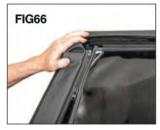
and zip it down a few inches (FIG 65). Repeat this on the passenger side of the rear window. You may have to lift the quarter window up to secure this second zipper. Once both side zippers are secure, zip the rear window zippers down about half way (Fig 66). You will close these zippers completely at the end of the install.
