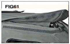
Locate the drivers rear quarter window. Line up the driver's side Quarter window to the zipper on the deck and zip it as shown in FIG's 59, 60 & 61 Repeat this on the passenger side of the vehicle.
