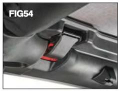
Step 9: Installing the Top Deck to the Jeep® With the header resting on the windshield, close the front header latches to secure the front of the top to the wind- shield. See FIGs 52, 53 & 54.
