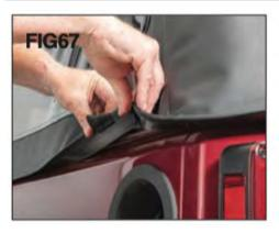
Step 10: Installing the Top to the Jeep Body
