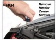
Step 1: Remove Existing Soft Top Fabric Put on safety glasses. After verifying that you have the correct factory original bow system and hardware, remove the existing soft top from the vehicle.
