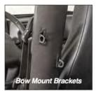
The roll bar mounted Bow bracket stays on the vehicle.
