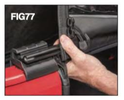
After sliding the retainer all the way through the "C" Channel, roll the tailgate bar into the mounts with the outside of the fabric facing towards the rear of the Vehi- cle (Figs 76 & 77).
