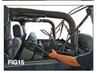
Un-latch the over door bow from the roll bar mount bracket and the rear bow from the Bow mount bracket (Figs 13 & 14).
