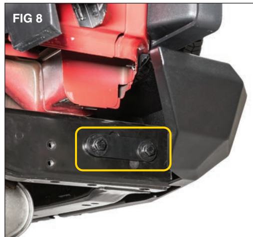
While holding the bumper support plates in place, thread the 12 x 40mm Bolts (A), lock washer (D), and flat washer (C) through the plates, frame rail and into the bumper using a 18mm socket. (FIG8)
