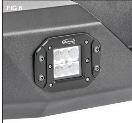
Flush Mounted Reverse Lamps: If installing flush mounted “Cube” style lamps, mount them as shown, using the 6mm Button Head bolts (B). (FIG6)
