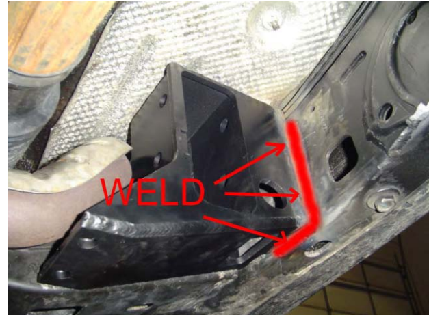
D.S. Bracket Welded in Place
