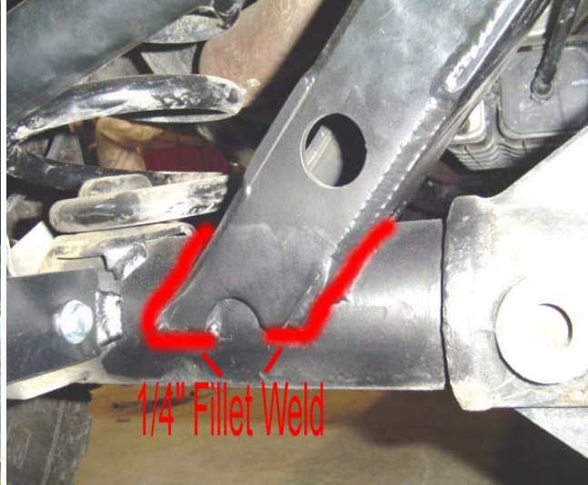
Welding the rear cradle
