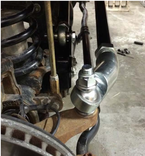
Passenger side knuckle connection
