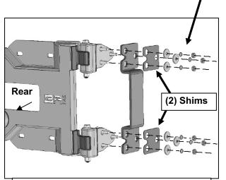
(Fig 16) Attach Inner Hinge Reinforcement Bracket and Shims to end of Hex Bolts
