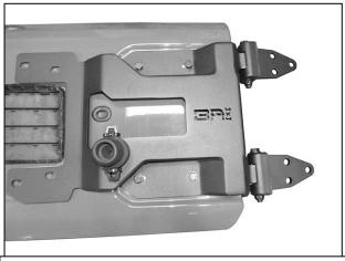
(Fig 10) Attach Door Reinforcement to rear door
