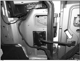
(Fig 4) Remove plastic panel from passenger/right side of cargo area. Release door check rod (arrow) and remove bolts from hinges to remove rear door
