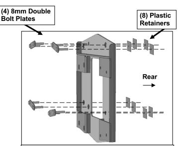
(Fig 18) Insert Double Bolt Plates through back of Offset Tire Mount Bracket. Secure Bolt Plates to Tire Mount with Plastic Retainers
