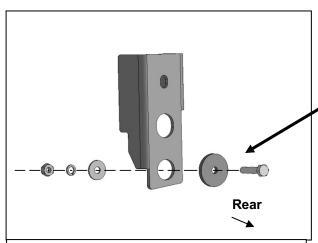
(Fig 22) Attach the driver/left Light Relocation Bracket to the top of the factory tire mount
