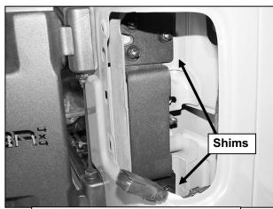
(Fig 17) Inner Hinge Reinforcement Bracket and Shims installed
