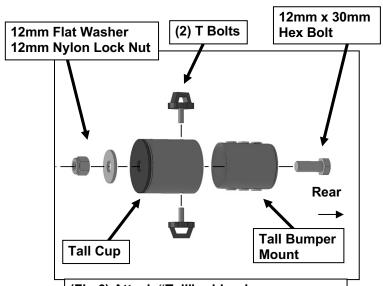
(Fig 6) Attach "Tall" rubber bumper Relocation Cup and Mount to bumper hole in driver/left side of rear door (figure 7)
