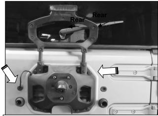
(Fig 2) Release rubber grommet (left arrow) and pull harness through hole in tailgate. Remove spare tire mount from rear door (arrow)
