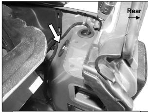
(Fig 13) Remove bolt (arrow) to remove passenger/right taillight assembly
