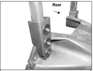
(Fig 25) Attach left and right Light Relocation Brackets to top of factory tire mount
