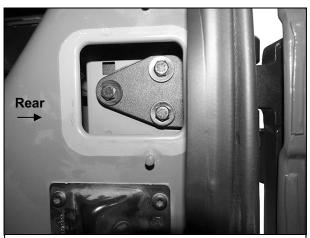
(Fig 12) Attach door hinges on Reinforcement assembly to body (top hinge pictured)
