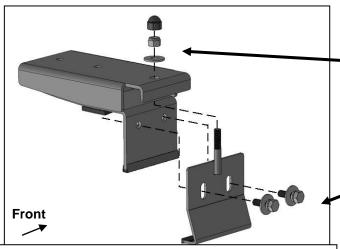
(Fig 3) Attach Clamp Bracket to Mounting Bracket
