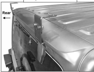
(Fig 7) Rear Window Bracket installed on passenger/right side
