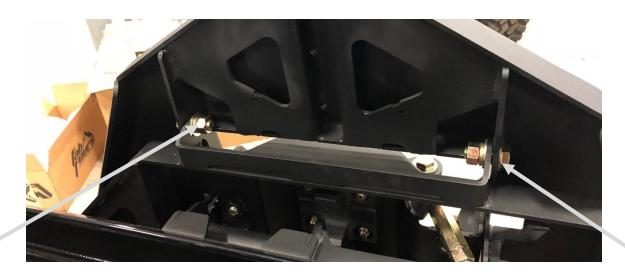
19. Use the ½" bolts washers and nuts and bolt through the cradle to the swing arm brackets. (At this point you can chose the desired angle you would like the tire carrier to sit at). Thoroughly tighten all bracketing and mounting bolts at this point.
