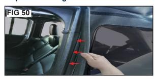
As shown in FIG's 50 & 51, roll the vertical plastic strip into the door surround slot securing it to the door surround. Next, starting at the driver's side front, attach the side belt rail into the vehicle body by "rolling" the plastic into the slot (FIG's 52 & 53).
