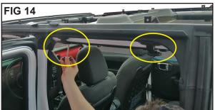
Line up the rear door surround bracket holes with the vertical holes in the rear horizontal roll bar. If you use a rolling motion while you push the brackets on it will be easier to install. Slip the two knobs through the brackets holes in the rear door surround (FIG 14). Loosely tighten the knob securing the rear door surround.
