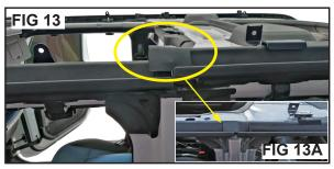
Line up the rear end of the front door surround with the front of the rear door surround as shown in fig 13 & 14. Make sure the rear door surround seals are on top of the front Door Surrounds as shown in Fig 13A.
