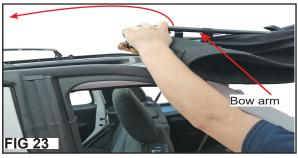
The bow arms will install to the front bow mount brackets located on the top of the door surrounds. With the help of a friend, lift each of the bow legs over the bow mount bracket (Fig 24).
