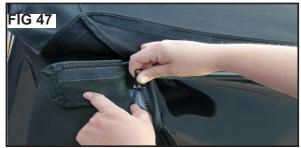
Locate the drivers rear quarter window. Line up the driver's side Quarter window to the zipper on the deck and zip it as shown in FIG's 43 & 44. Repeat this on the passenger side of the vehicle.
