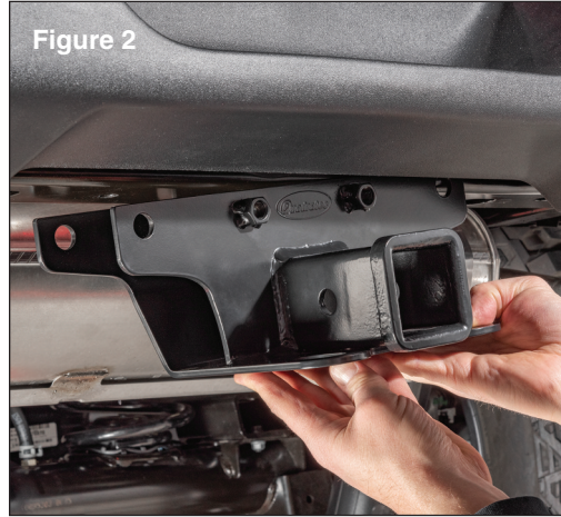
Slide the hitch in place over the cross member and align the holes in the hitch with the holes in the cross member. (FIG2)
