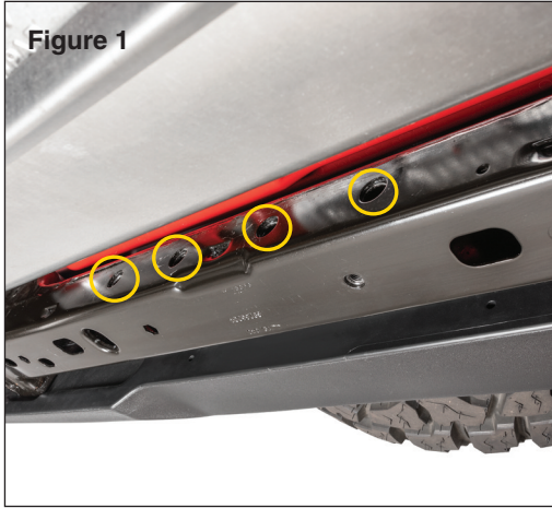
Put on safety glasses. Locate the 4 holes in the rear frame cross member. (FIG1)
