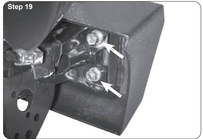
Secure the bolts with the 8 M12 nuts, split washer and flat washers on the back of the frame. Tighten with an 18mm socket and ratchet. (Step 19)
