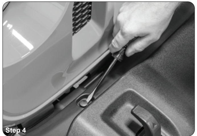
Step 4 Remove the plastic retainers using a small flat blade screwdriver. (Step 4)
