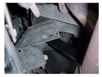
**Step 5:** Take the strut rod and attach it between the motor mount and the skid plate. Use one 3/8-16 bolt, lock washer, and nut to bolt it to the front of the skid plate and use the remaining <sup>1</sup>/<sub>2</sub>-13 bolt, washer and nut to attach it to the rear of the motor mount. The view in the photo is from the rear on the driver's side.
