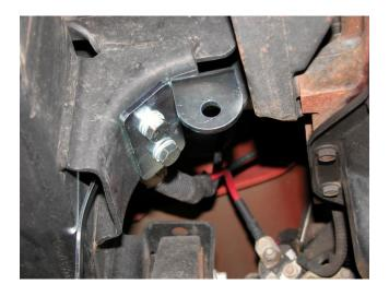
**Step 3:** Repeat steps 1 and 2 on the passenger side motor mount. On the passenger side, the T-shaped nut plate is more easily inserted from the bottom of the motor mount as shown above. The view above is from the front. **NOTE:** On the passenger side the tab MUST be towards the front of the vehicle.
