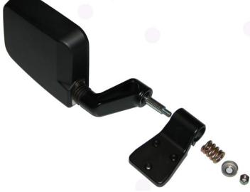
Step 4: Mount the mirror into the new relocation bracket using the cup washer and nut. Position the mirror and tighten the nut.
