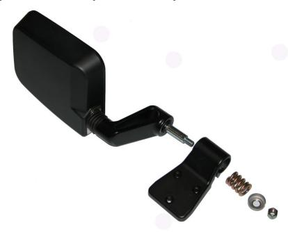
**Step 4:** Remove the original mirror mounting bracket from the door.
