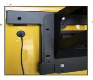
STEP 1 Remove (2) driver-side bolts from the Spare Tire Carrier
