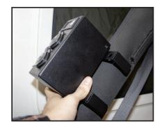
Position the Power Panel in the desired location along the roll bar.
