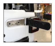
Remove the torx bolts connecting the stock tailgate hinge to the tailgate.
