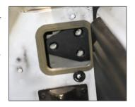
Remove the bolts connecting the stock hinge to the tub of the Jeep through the interior access panel.
