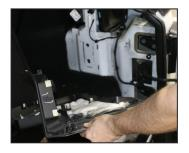
Remove the plastic cover over the hinge access hole.
