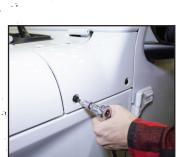
Using a T40 Torx bit, remove the 2 bolts on the side of the Jeep that fasten
