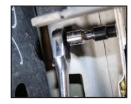
Using a 10mm socket, remove the nuts (6) that hold the nerf bar to the pinch seam on the underside of the Jeep.
