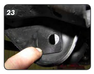
d. Re-install the control arm to the axle with the factory bolt with cam lock washers. Rotate the cam lock so that the bolt will be as far back in the slot as possible (most rearward setting = max caster). Snug the cam hardware so that the cams are retained within the stops. Final torque will be completed with the weight of the vehicle on the suspension. [2]
