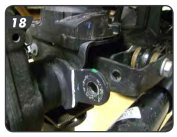
r. Install the shorter passenger side post on the side of the track bar mount at the sway bar link mount location with it pointing outboard [19]. Fasten with the ½" nylock nut and tighten to 65 ft-lbs.
