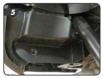
i. Support the axle with a jack under the center of the differential and remove the shocks from the frame and axle (18mm), save hardware [6].
