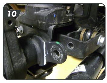
Install the shorter passenger side post on the side of the track bar mount at the sway bar link mount location with it pointing outboard [11]. Fasten with the ½" nylock nut and tighten to 65 ft-lbs.
