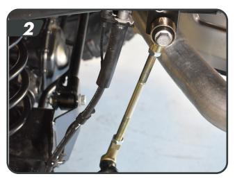
d. Install the rear bump stop spacers on the axle. Fasten the bump stop spacer to the axle with the 5/16" x 7/8" bolts, nuts and washers. Torque bolts to 20 ft-lbs. (½") [3 - 3" extension shown]
