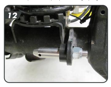
The kit comes with disconnect retention brackets to hold the links when the links are disconnected. Install the retention brackets using the provided 5/16" bolts into the factory hole in the front of the coil bucket [13]. These are designed to slightly interfere with the edge of the coil bucket to hold them in place.
