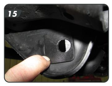
Re-install the control arm to the axle with the factory bolt with cam lock washers. Rotate the cam lock so that the bolt will be as far back in the slot as possible (most rearward setting = max caster). Snug the cam hardware so that the cams are retained within the stops. Final torque will be completed with the weight of the vehicle on the suspension. [16] Note: Use of a jack on the axle may help to align the cams. Wait for final cam placement until the other side is complete.
