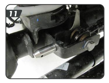
Install the longer disconnect post on the driver side axle sway bar link mount with it pointing inboard [12]. Fasten with the ½" nylock nut and tighten to 65 ft-lbs. Tighten the post with the pin hole parallel to the ground. Slide the polyurethane spacer on the pin up against the axle tab.
