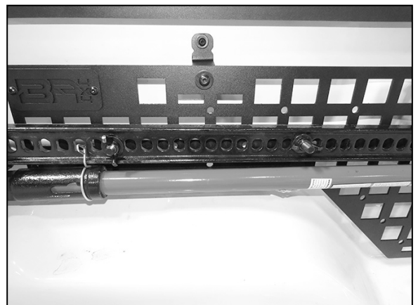
(Fig 8) Example of beam style recovery jack attachment to Carriage Bolts in Panel (arrows)
