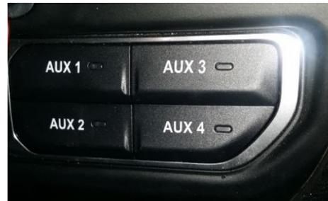
Figure 15: OE Upfitter Switches
