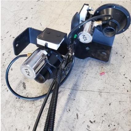
Figure 7: JT220 Horn Driver Prewire and T-Fitting
