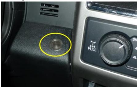
Figure 14: Horn Button Installed in Dash
