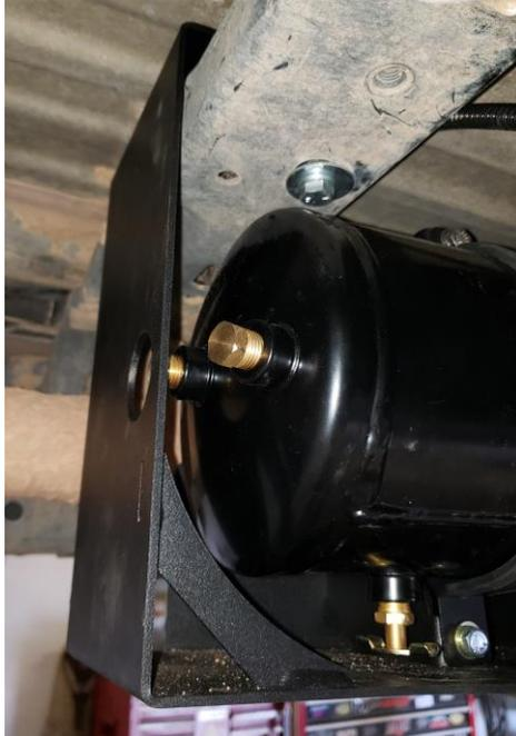
4. Use [H7](#), [H9](#), [H10](#), [H11](#), [H21](#), & [C4](#) to secure the back of the compressor mounting plate to the front crossmember. Use any hole in crossmember that is accessible. ([C4](#) not shown)
