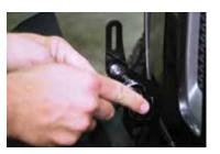
4. Line up the groove on the extension with the bracket itself. Then secure it using the included hardware and a 10mm socket.
