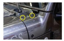
1. On either side of the vehicle, remove the two factory bolts as indicated using a T40 Torx driver.
