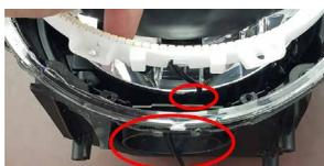
5. Route the wire through the hole at the bottom of the headlamp. Then return the retainer to its original position.
