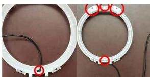
4. Route the wire through the small hole at the bottom of the light pipe retainer. Set the RGBW DRL halo in place. The tabs on the halo should line up with the slots in the retainer. Then re-pin the JST connector.
