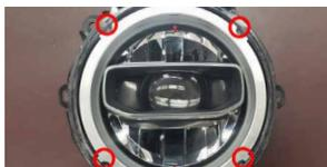
1. After opening the headlights, remove the four T20 torx screws holding the silver outer shroud in place. Remove the silver shroud.
