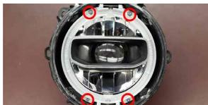
2. Remove the four T20 torx screws holding the light pipe retainer in place. Remove the retainer and light pipe.
