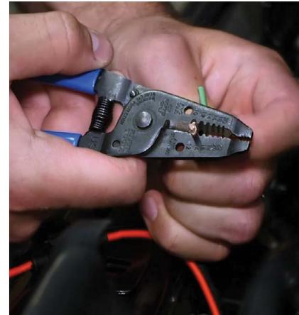
7. Locate and connect to one of the four power wires for the Auxiliary Switch Bank near the battery. Using wire strippers, remove enough insulation to make a good connection. Insert the yellow wire into the butt connector and crimp it to secure the connection.
