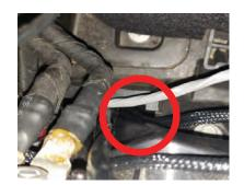
7. Route the harness output wire through the small opening in the engine bay to the passenger wheel well, located between the battery and the passenger fender.
