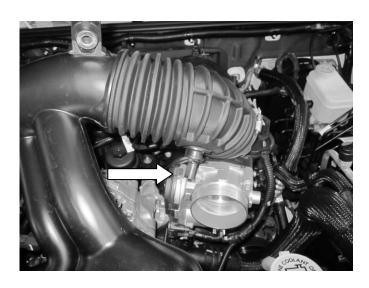
**g)** Depress the clip to release the electrical connector from the IAT sensor then remove the air inlet hose from the engine bay.
