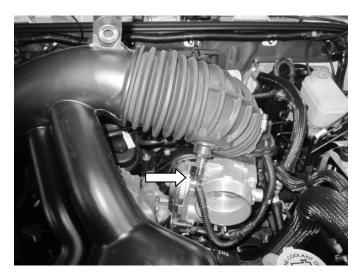
**f)** With the two M6 bolts removed, lift the air inlet hose up to reveal the IAT sensor and harness.
