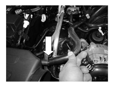
**h)** Disconnect the valve cover breather hose from the air box.
