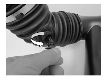
**I)** Remove the IAT sensor from the factory air inlet tube. Gently twist and pull out the sensor.
