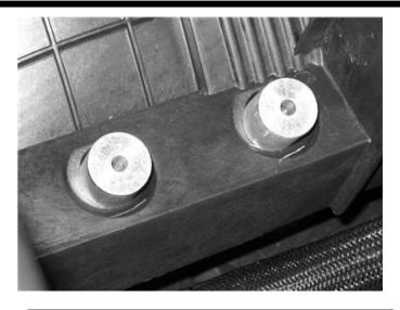
**f)** Place the two supplied spacers in the same location you removed the stock grommets from.
