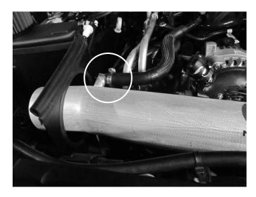
**I)** Attach the stock breather hose to the breather tube on the intake tube and secure with the supplied #12 hose clamp.
