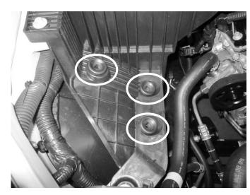
**j)** Remove the three rubber grommets - just squeeze and pull.
