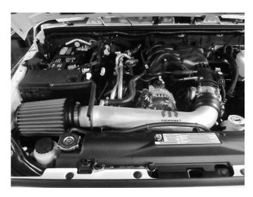
**n)** MOPAR Cold Air Intake installed on vehicle without the engine cover.
