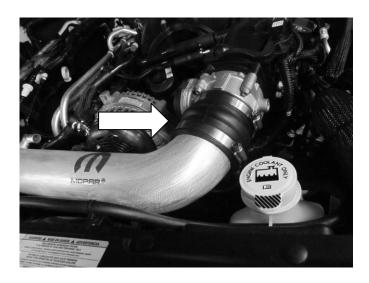
I) Attach the end of the MOPAR intake tube with hump hose onto the throttle body. Slightly tighten the hose clamps.
