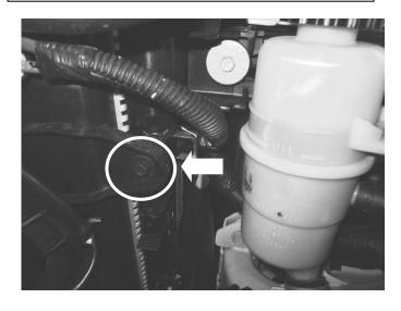
**k)** Loosen and remove the M6 screw securing the radiator fan shroud. The bolt will be reused in the later steps.
