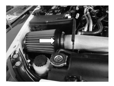
**m)** Finally, Install the MOPAR dry media filter onto the MOPAR intake tube. Slightly tighten the hose clamp.
