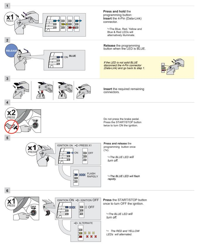
Once you have the alternating red and yellow LED's, unplug all the connectors from the remote start brain. Be sure to disconnect the 4-pin black data link plug last.
