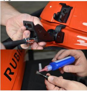
Completely unscrew the adjustment bolt, removing the top portion of the latch. Apply threadlocker to the threads.
