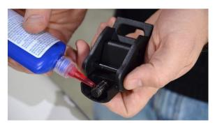
Completely unscrew the adjustment bolt, removing the top portion of the latch. Apply threadlocker to the threads.
