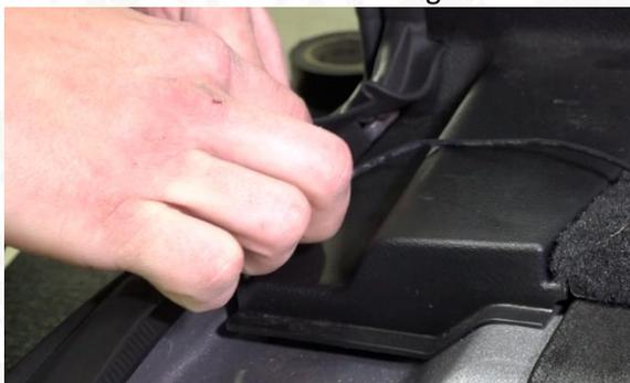
Push the conduit through the rubber seal illustrated in Step #2 and pull it through to the driver's side taillight.
