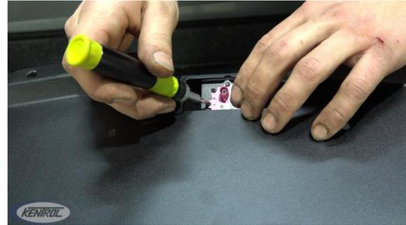
Push the third brake light and backside wires through the rear vent.
