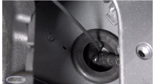
Using a body clip removal tool, pull the OEM license plate light connector and route it through the driver's side light cavity.
