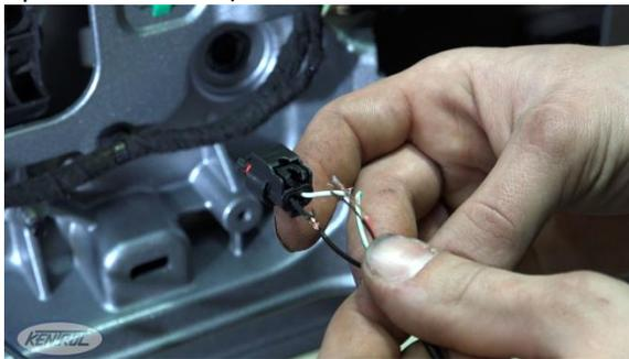
With the long Backside wire, run it through the tailgate wrap, make sure there is an inch or two of slack so the wires are not stressed excessively when the Tailgate opens.
