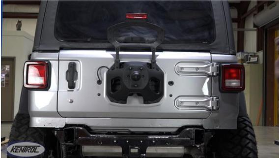
Using a T-40 Torx wrench remove your spare tires retaining clip. Next remove the three lug nuts and remove the vehicle's spare tire.
