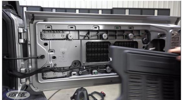
Using a flat head screw driver open the drivers side taillight access panel, remove the plastic bolt using a T-40 Torx Bit.
