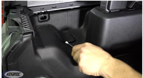
Using a flat head screw driver, pull away the driver's side inner panel enough to fit your arm. \*If you choose to hide your wiring, use a pair of scissors to carefully make a cut into the tailgate fabric cord wrap and push wiring through.
