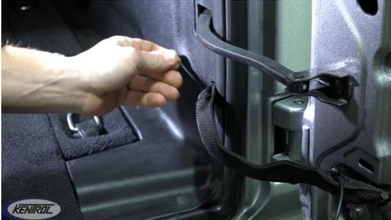
Make a cut into the rubber conduit seal just above the driver side taillight. (NOTE: Wires will be pushed through later)
