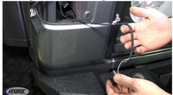
Strip the license plate connector wires and connect to the longer Backside cables: Red to white and black to black. Make sure these connections are properly insulated. Push the wires back into the taillight cavity.
